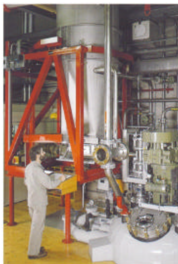
Chemical feed to reaction vessel by a Gericke loss-in-weight feeder.
