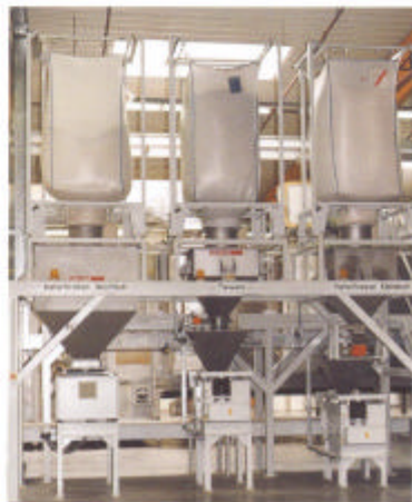
Muesli ingredients are discharged from big bags into a continuous feeding/mixing line.
