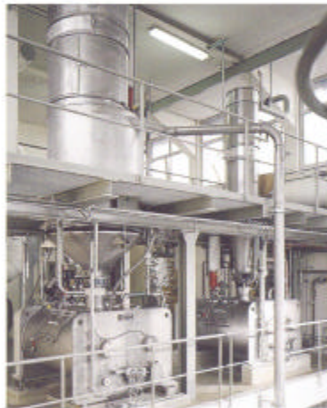
Ploughshare mixer plant for the pre-mix of confectionery ingredients
