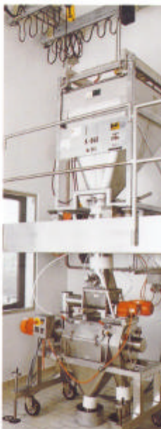
This chemical production dense phase conveyor incorporates weighing and recording of the throughput.
