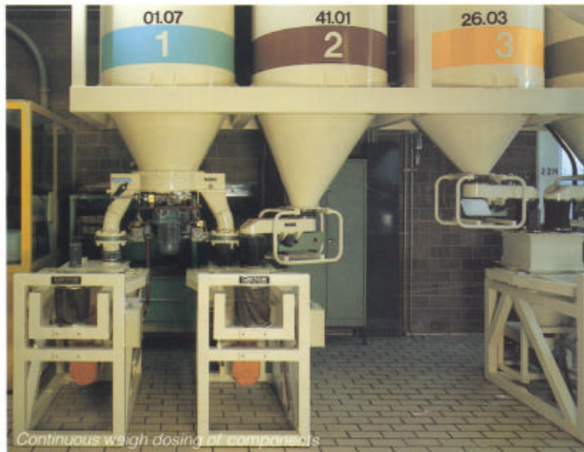
Process control by microprocessor controlled continuous weigh feeders and mixer.
