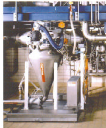
Chemical products: Pneumatic dense phase conveying with weighing and throughput recording.
