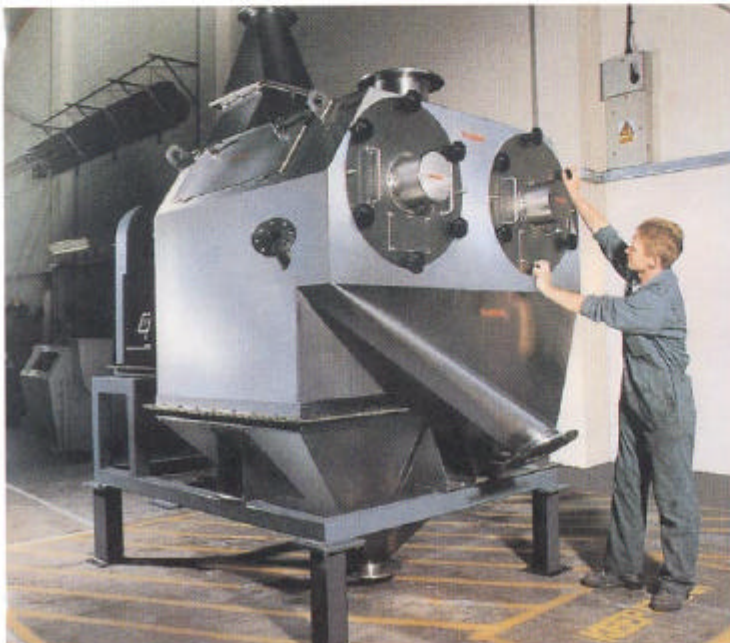
Special CSM 1542 Twin Sifter on final assembly
