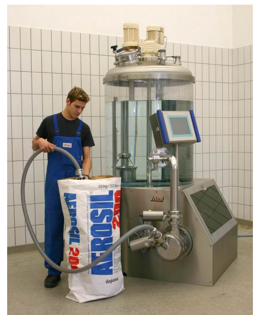
Pict 1.: Dust free powder induction with TDS induction mixer
