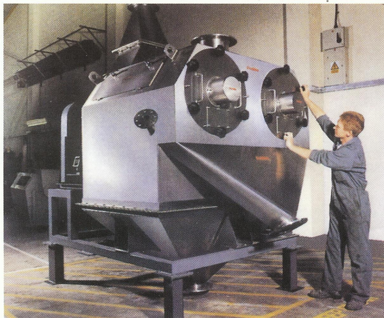
Special CSM 1542 Twin Sifter on final assembly
